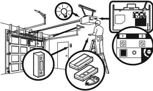
1. Press and release the “learn” button on the motor unit. The learn indicator light will glow steadily for 30 seconds.
